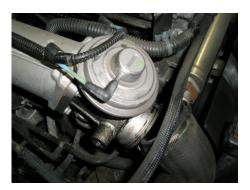
Disconnect the vacuum pipes from the EGR assembly and connect them together as shown by removing one rubber end.
