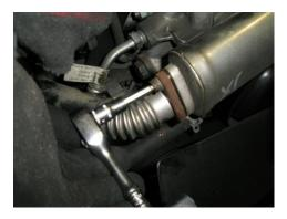
Remove the EGR assembly at the water jacket on the front of the cylinder head and at the inlet manifold.
